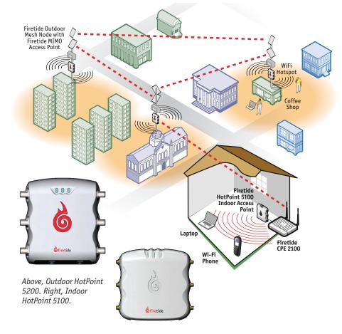
Wi-Fi access to any indoor or outdoor location without the need for backhaul cabling. HotPoint access points can also connect directly to a conventional wired infrastructure eliminating the need to install a mesh node in locations where wired connectivity is readily available.
